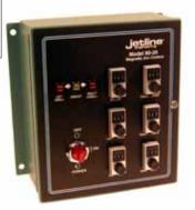
Magnetic arc control provides even heat distribution, prevents undercutting, eliminates excessive porosity, ensures sufficient penetration, and evens out the weld puddle. Combined with a magnetic probe, a magnetic field is created around the arc to precisely position, oscillate, and stabilize it.
