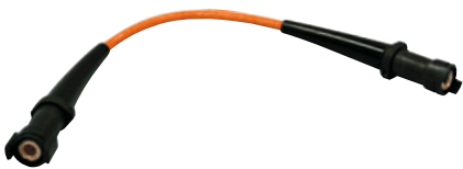
Series Cable Adapter 195437 Used in series/parallel arrangement to power four blankets/air-cooled cables to create extra heating area. The series/parallel arrangement requires four equally sized blankets/air-cooled cables, two output extension cables and two series cable adapters.
