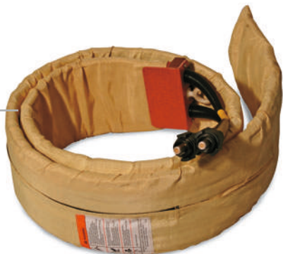
Induction Blanket The flexible, lightweight induction heating blankets come in a variety of sizes and are capable of preheat temperatures up to 400 degrees Fahrenheit (204°C). The blankets easily conform to circular and flat parts and install in a matter of seconds. Manufactured from durable high-temperature materials, flexible induction blankets are designed to withstand the tough conditions in both industrial and construction applications. See ordering information on the back page for available sizes.
