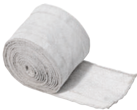
Preheat Cable Cover 204611 30 ft. (9.1 m) 204614 50 ft. (15.2 m) 204620 80 ft. (24.4 m) Used in preheat applications to protect the heating cable from slag and molten metal created during welding. The 1/2-inch thick preheat insulation must be used with the preheat cable covers.
